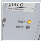
The automatic oil injection system lubricates the cutting shafts when shredding and guarantees a constantly high shred performance.
